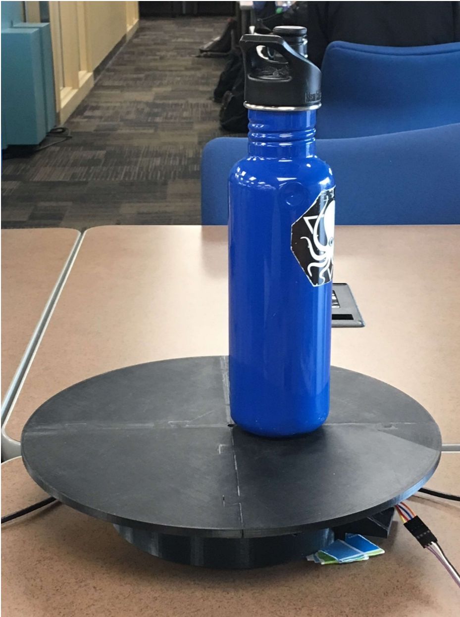
Figure 3: Scan platform with cylinder used for calibration purposes
